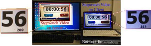
Fig. 13. Testbed for measuring delay.
