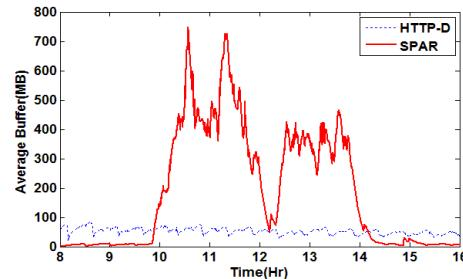
Figure 4. Average user buffer level for HTTP-D and SPAR
