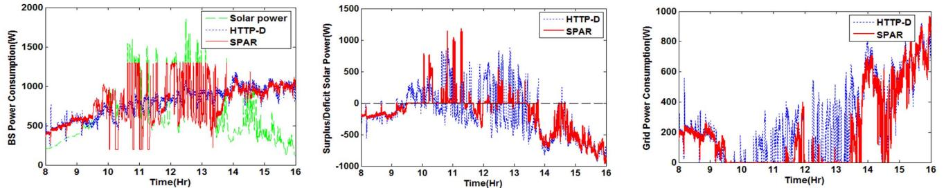
Figure 3. (a) left, solar power and BS power consumption for HTTP-D and SPAR (b) center, surplus/deficit solar power due to HTTP-D and SPAR (c) right, grid power consumption for HTTP-D and SPAR
