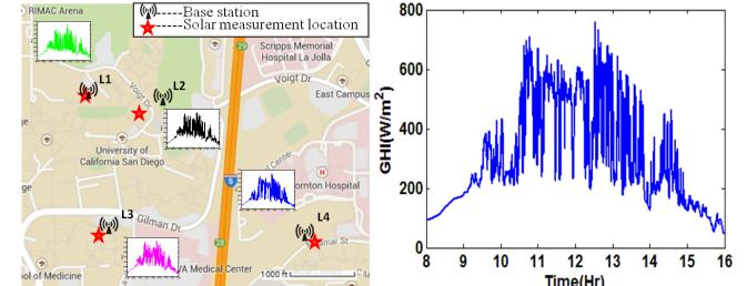
Figure 1. (a) left, Map showing locations of 4 BSs and nearby solar irradiance measurement, (b) right, solar irradiance at L1 on Dec. 11, 2014 between 8AM-4PM
