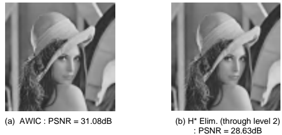
Fig. 6. Comparison of image quality after AWIC and H* elimination techniques using the Lena 512x512 grayscale image sample.
