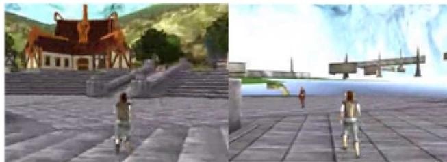
Fig. 11. Comparison of video frame quality for different rendering setting with 300 kb/s encoding bit rate. Left: view distance =150 m. Right: view distance = 70 m.
