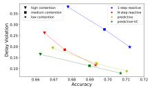
Figure 6. Delay violations vs avg. accuracy for different model selection methods under different contention levels
