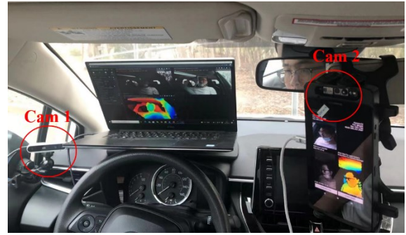
FIGURE 2. Facial expression data collection set-up using multiple cameras in vehicle
