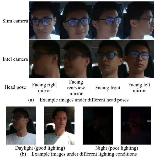
FIGURE 3. Example images captured by two cameras under different (a) head poses and (b) lighting conditions
