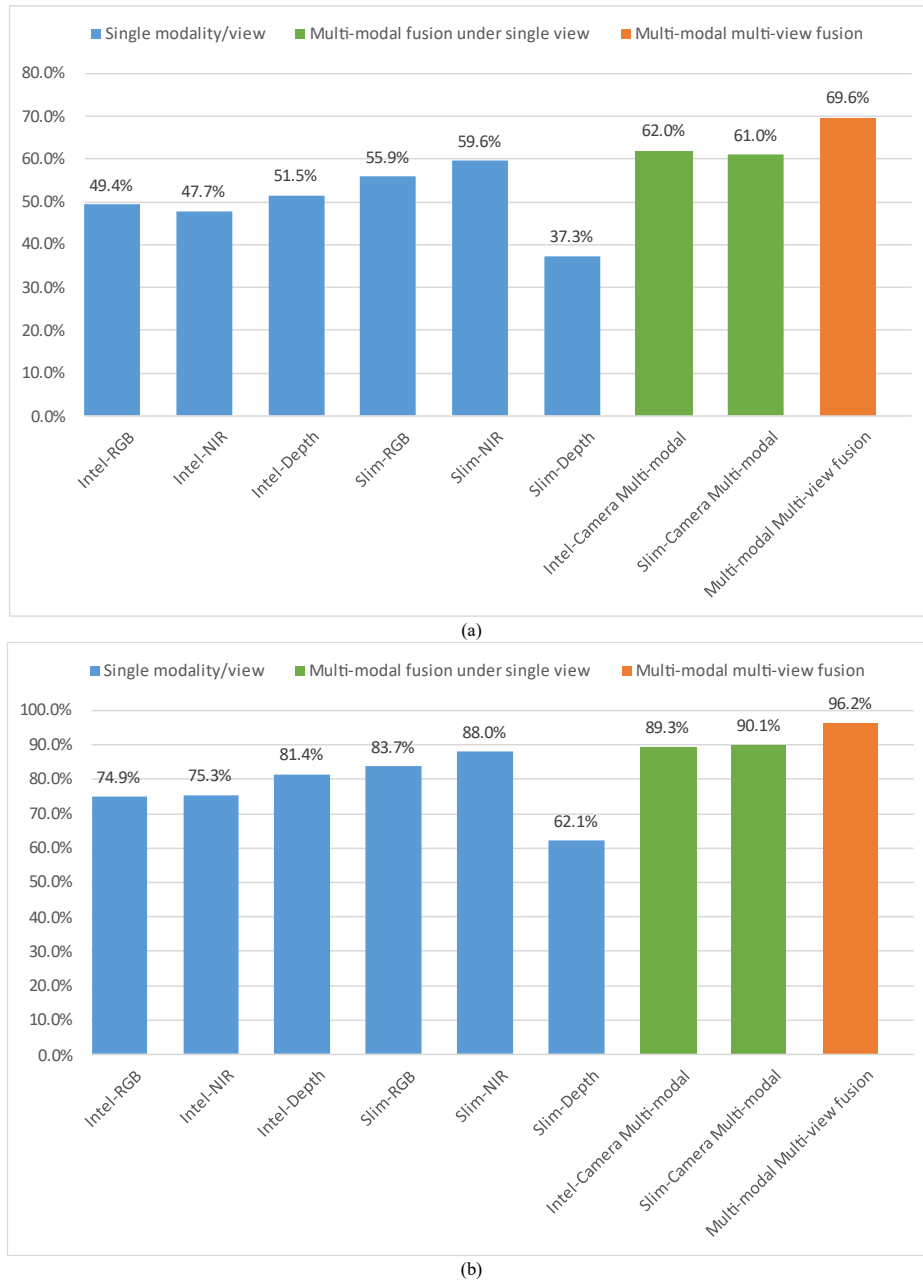
FIGURE 13. Overall Recognition Accuracy Results Plot of Single Modality, Multi-modal Fusion and Multi-modal Multi-view Fusion on Vehicle Data (a) General Case (b) Driving Case
